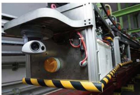
Figure 1: Rail-based robot system TIM in the Large Hadron Collider (LHC)
