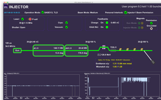
Figure 3: Status screen for the injector section of the European XFEL linear accelerator created with JDDD.
